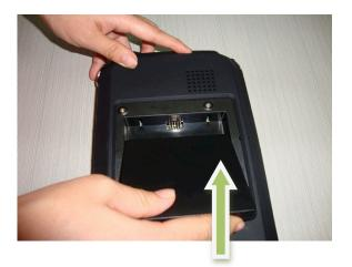
Push the battery into the battery compartment.
